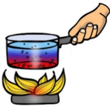
The cooler water particles drop to the bottom of the pot and take the place of the heated ones. So, the heat transfer is taking place because of the movement of the warm particles.
