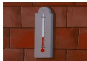
When something gets hotter it will expand, or get bigger. At the same time, when something gets colder it will shrink. This property is used to make mercury thermometers. The line in the thermometer is actually liquid mercury. As the liquid gets hotter, it will expand and rise in the thermometer to show a higher temperature. It's the expansion and contraction due to temperature that allows the thermometer to work.
